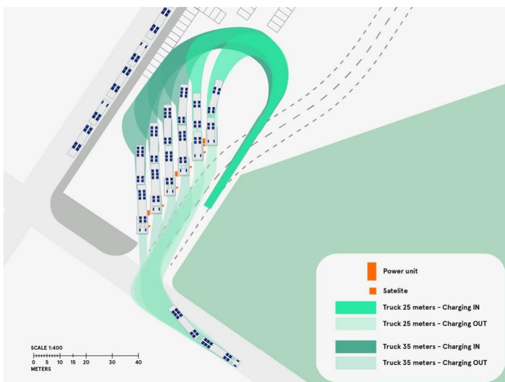
Figure 23 Analysis of turning circles of various truck configuration in design phase can be seen as best practice. This image is from Jula Logistics site in Falköping. Image from REEL- Charging infrastructure for trucks (CLOSER, 2024).
