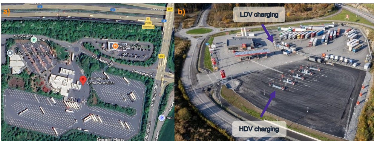
Figure 11 A typical layout for a B1 rest area a) Aral Autohof Porta Westfalica, Germany, with many parking spots for trucks. Image from Google maps. b) Circle K Vädermotet, Sweden, with charging for both LDVs and HDVs which are separated. Image from Circle K.
