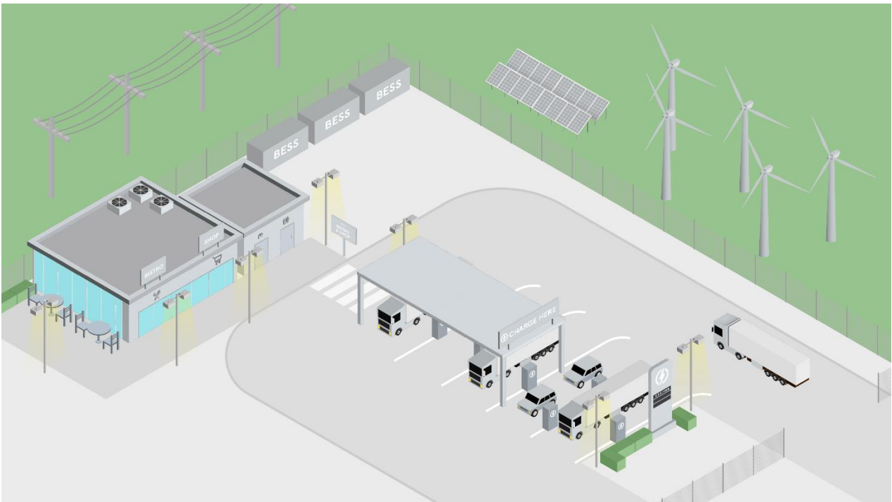
Figure 1 A schematic hub design including elements from the four different subsystems: Vehicle related, Human related, supporting information and Energy supply which are highlighted in the following figures.
