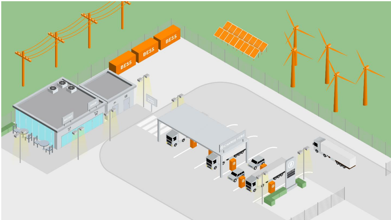
Figure 5 Illustration of a schematic hub design with the energy supply subsystem highlighted in orange.
