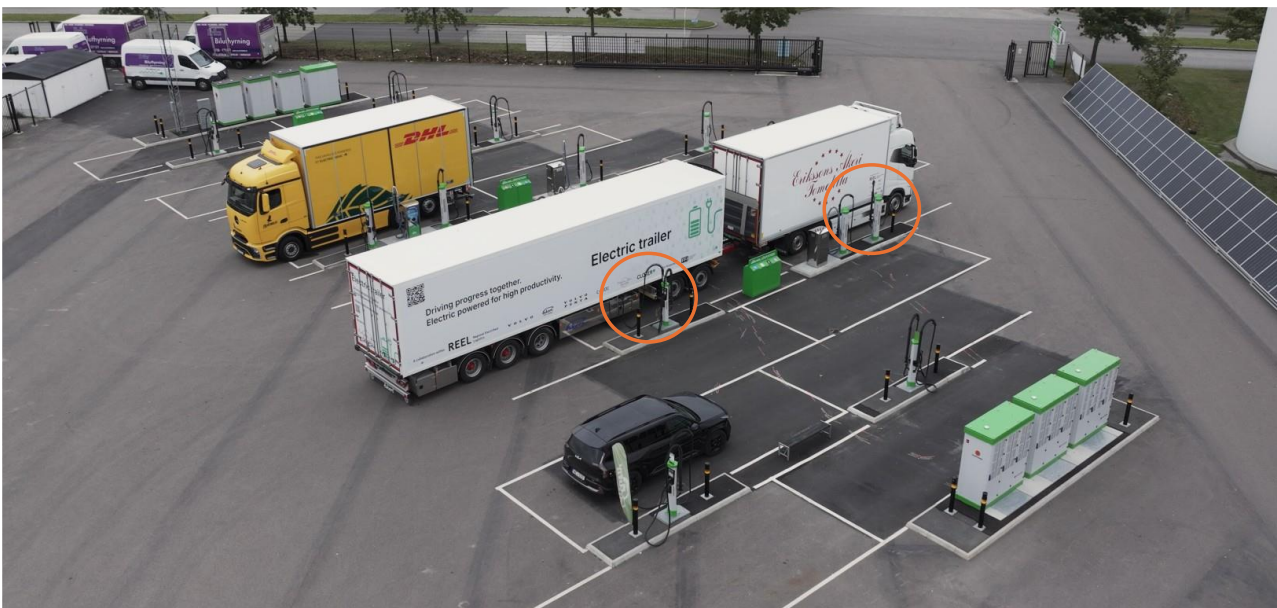
Figure 24 Charging session with e-trailer at the Rifil station in Malmö. Image from CLOSER.
