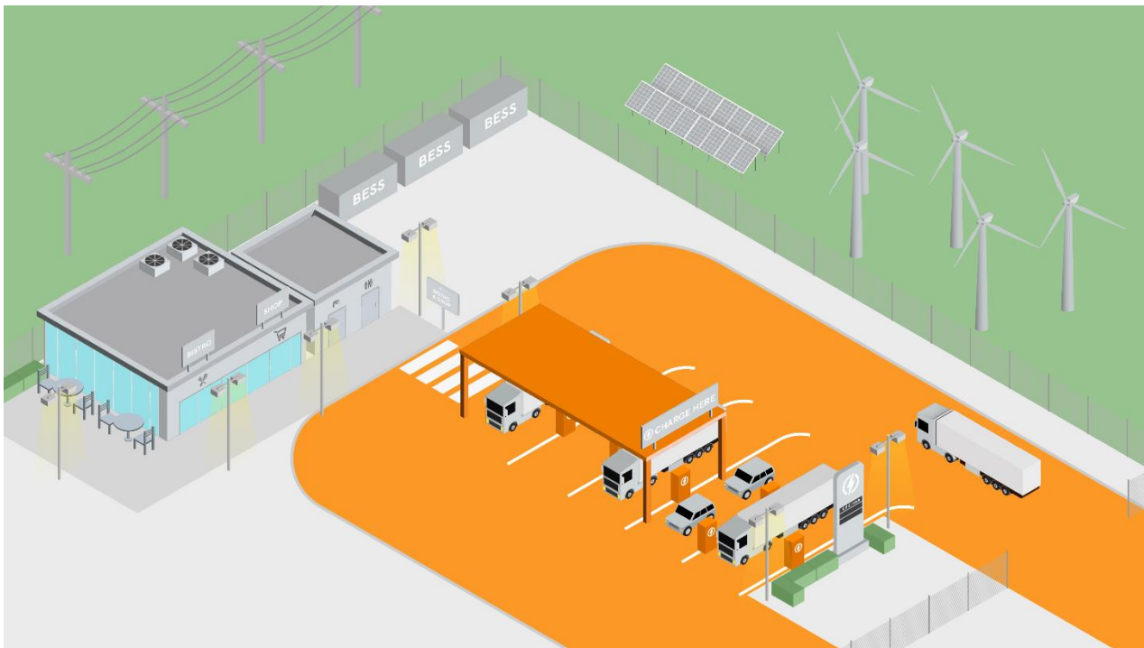
Figure 2 Illustration of a typical hub design with the vehicle related subsystem highlighted in orange.
